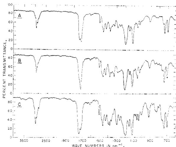
Fig. 1.—Infrared absorption spectra: A, mixture of *cis*- and *trans*-1-benzyl-2-carboisopropoxy-3-methylethylenimine; B,  $1718\text{ cm.}^{-1}$  ethyleneimine; C,  $1736\text{ cm.}^{-1}$  ethyleneimine, all as pure liquids.
